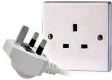
These are the modern plugs that are also used in Malta and have a fuse in the plug connected to the equipment. The pins are rectangular and the earth one is bigger, longer and thicker and does not have insulation like the other pins. Normally wall sockets have switches. Wires are **LIVE RIGHT, NEUTRAL LEFT**.
