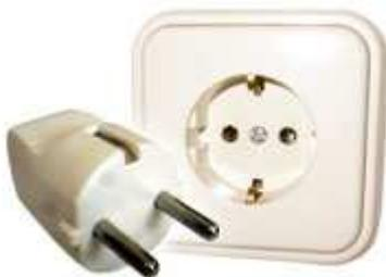
This plug and wall socket are like type E except that the earth contact is made by side contacts instead of pins. This is known as Schuko from the invented German word "Schukostecker" that means "protective contact plug". This plug allows the possibility that the live and neutral wires be swapped and are therefore not polarized. This F wall socket also accepts plugs C u E.
