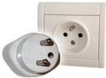
This type of plug and wall socket are French. Note that the earth pin is in the wall socket while the plug connected to the equipment has a hole where the earth pin makes contact. The pins are spaced 19 millimetres.
